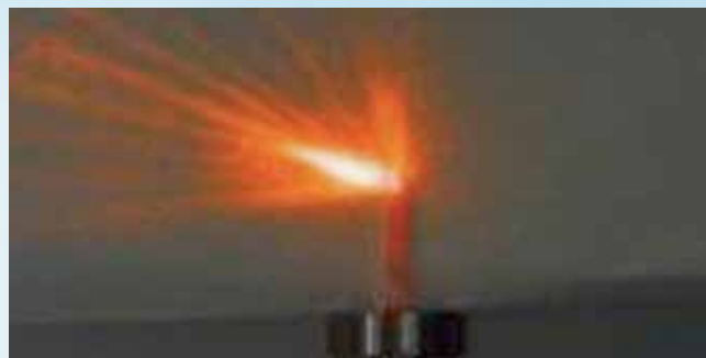
100% deflection of the laser beam by the prism.
