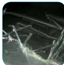
Presence of fibres in everX Posterior increase the adhesion by providing mechanical retention University of Turku, Finland, 2013 magnification x16
